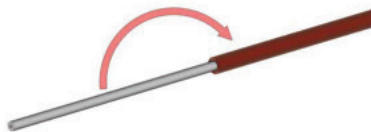
Fold back shield braid over jacket
